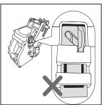
If the hook is still in the lower position, this means it has not been correctly positioned.
