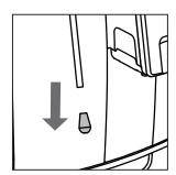
Clean the steam wand with a damp cloth. To clean it more thoroughly, you can unscrew the nozzle and wash it with running water.
