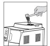
1 Lift the lid of the pre-ground coffee compartment and add one level measuring scoop of pre-ground coffee.
