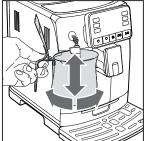
6 When the milk froth comes to the desired consistency. Press the **START/STOP □** button to stop steam dispensing.
