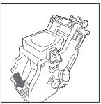
Make sure that the lever is in contact with the base of the brew group.
