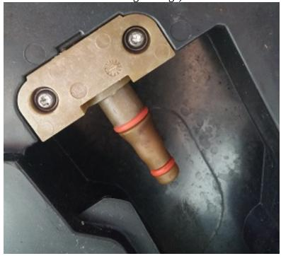
2. Remove the Torx screws and pull down the visible portion of the valve. You will be left with this:
