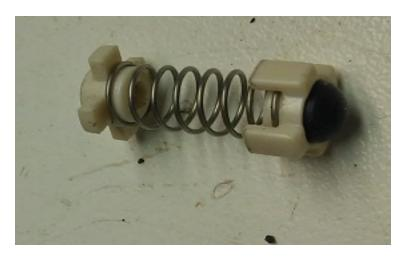
5. Once the valve is out, gently pull the spring off of the upper component and remove the black ball.
