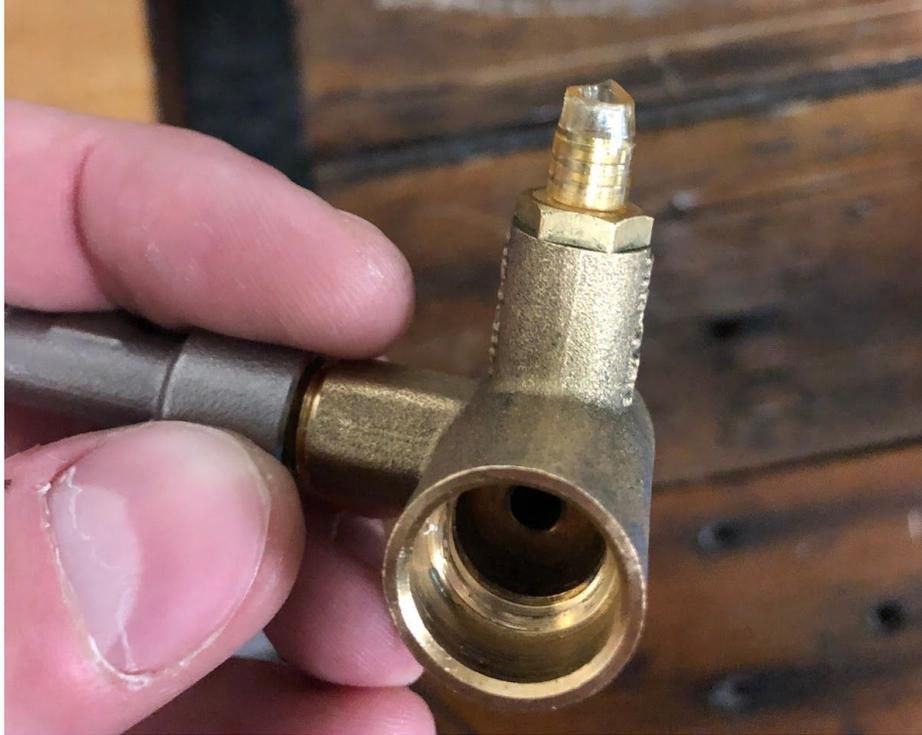
**If your machine has this, do not remove it. It is needed for the silicone tubing you are removing to seal onto the nipple fitting appropriately.**
