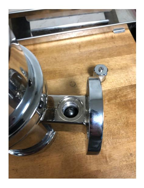
If you tip over the group, the ball will fall out - **do not lose this**. Underneath is the nut that acts as a channel for the water that lifts the ball:
