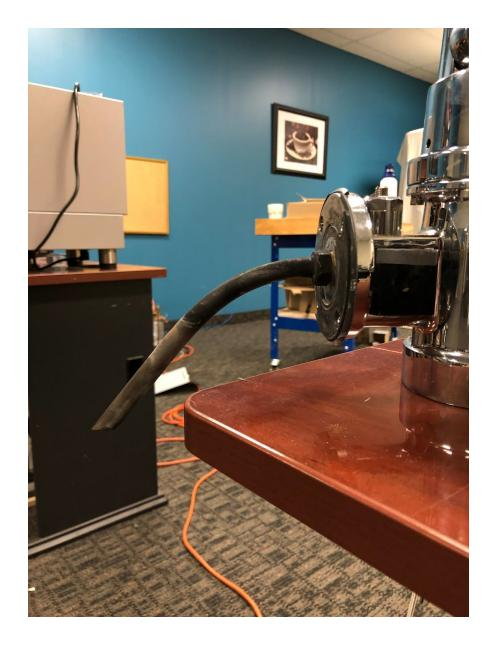
Once the group has been removed, you'll need to remove the dip tube. This piece is where the water travels through to make it to your group. To remove it, use your 19mm wrench on the nut portion of the dip tube that is close to the back of the group. **As mentioned in the notes, you may need to shock this part to get it break free**:
