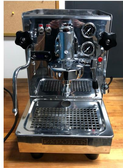
All of the screws on these machines are easily accessed from the outside. Expobar has some of the easiest casings to remove of any machine brand. You can start removing screws from any part of the housing, as it is all one piece. There is not a particular way they need to come off. So I will just highlight where the screws are (see photos on next page):
