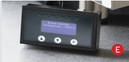
Fig E. The factory setting for the brew boiler temperature is 103°C
