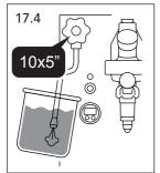
**Steam wand cleaning.** Fill a jug with 500 ml of cold water, add the content of 1 bottle of detergent liquid (I) and immerse the steam wand (5) in this solution. Open the knob (4) by turning it anti-clockwise and dispense steam for 5 seconds. Stop the function and wait for 5 seconds.
