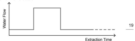
The graph shows an extraction where the flow is reduced both at the beginning (low flow START) and at the end (low flow FINAL) of the coffee extraction.
