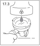
**Backflushing.** Insert the blind filter (D) into the filterholder and pour 1 bag of detergent powder (I) into the filter. Insert the filterholder in the group head (8) and lift the lever (13) for 10 seconds (Pic 17.2).
