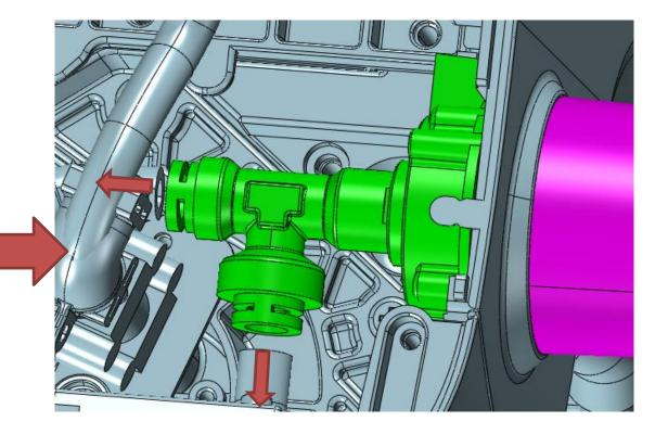
Remove clips, then pull out cables with quick coupling. Pay attention to the gaskets when removing the tubes because they will be used for the replacement steam valve
