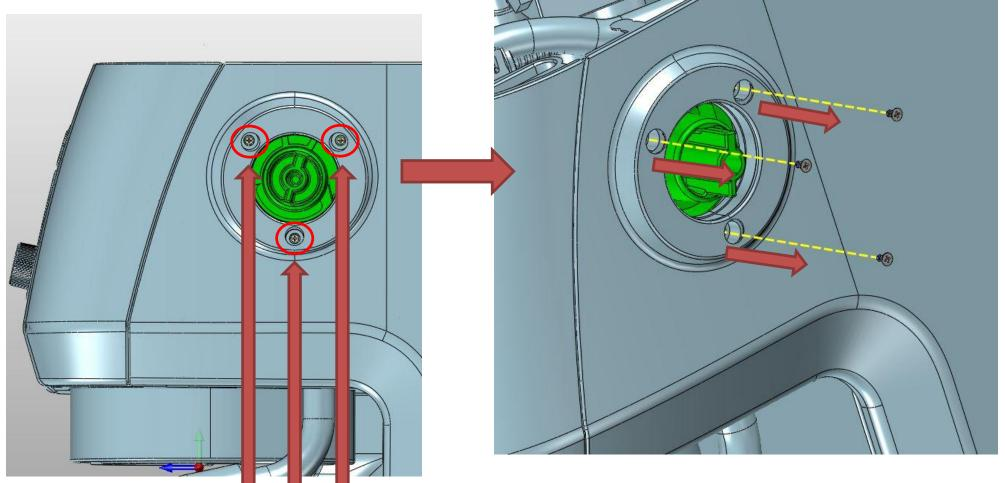
Unscrew and remove 3 screws of the right panel of the machine
