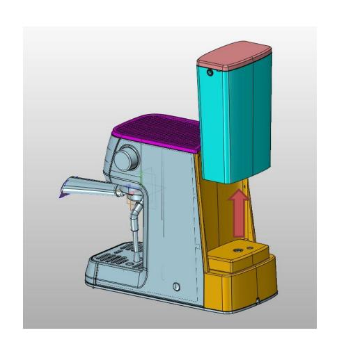
Remove the water tank, pulling it up
