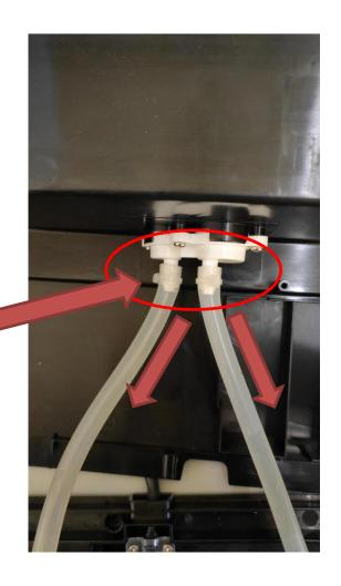
Remove the bands from tubes (cut them), then pull two tubes downwards
