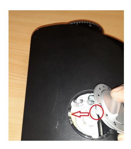
Put the knob back. The hook indicates the correct position.
