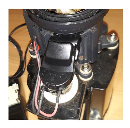
Replace the channel cover making sure that the hooks fit well.
