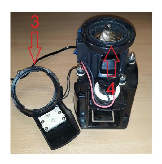
Pull the front panel (3) away while holding the selector for the fineness(4) in position.
