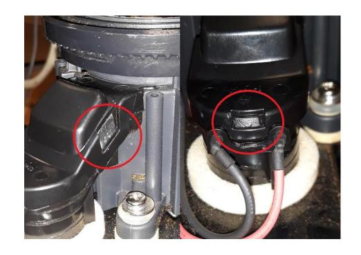
Remove the channel cover by unhooking at least two of the three hooks that hold it.
