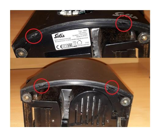
With the same tool, lever in the four circled points to release the housing.
