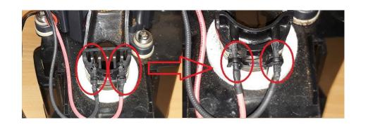
Pull the two ionizer needles out of the old holder, insert them into the new one and put the holder in place. Be sure to push the needles all the way through.
