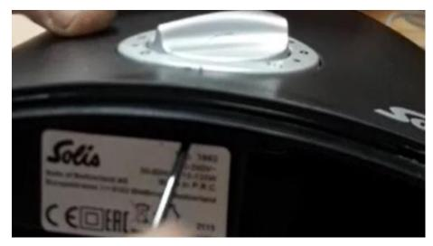
Insert a fairly long and thin object (for example a watchmaker's screwdriver) into the hole located under the base of the grinder, and press to be able to remove the knob.
