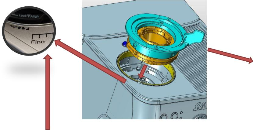
Align the sign on the machine lid and the grinder mechanism then lock the grinder the mechanism by turning it clockwise
