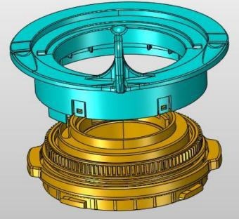
Turn the dial ring clockwise and lock it on the mechanism
