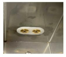
• If there is no water being sensed and the water is determined to have proper mineral content for conductivity then it is possible that one of the wires on the back side of the assembly has been disconnected.
