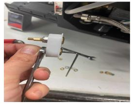
Note: the assembly has tension springs which will cause the contactor screws to push inward when seating the reservoir. It is important to ensure that the threaded posts are not touching the white housing during reassembly as this can cause the post to hang up and stay seated back away from the reservoir.
