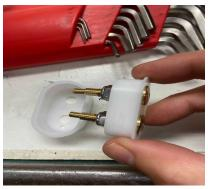
Use a 10mm wrench to hold the silver nut and the 2.5mm allen wrench to turn the screw counter clockwise to expose more of the contactor screw.
