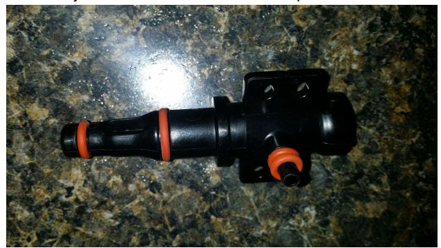
6. Next, using your flathead screwdriver, unscrew the top of the boiler spout. You'll see two little tabs that need to be aligned in order to lift it out. You may need to push the top part off by pressing on it from below with your screwdriver. Once this is apart, you will see a little, black rubber stopper, along with a spring.
