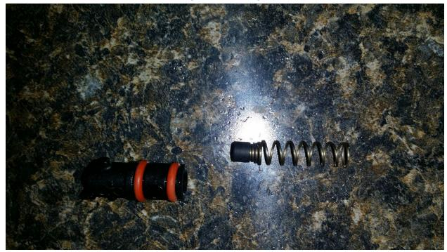
The little black plug you see in the photo is what causes the squeak. As it moves back and forth from the water pressure during the brewing process, it rubs against the inside of the plastic chamber.
