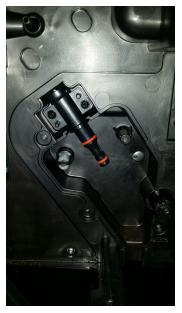
5. Remove the entire spout. Be careful, as there are 2 red o rings on the back side of this. If the o-rings come off and remain in the machine, use your allen key or a pick tool to hook them so you can remove them from the machine. The spout should look like this:
