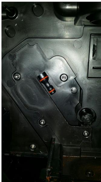
Remove the four screws using your 2mm allen key so that you can remove the panel covering the boiler spout.
