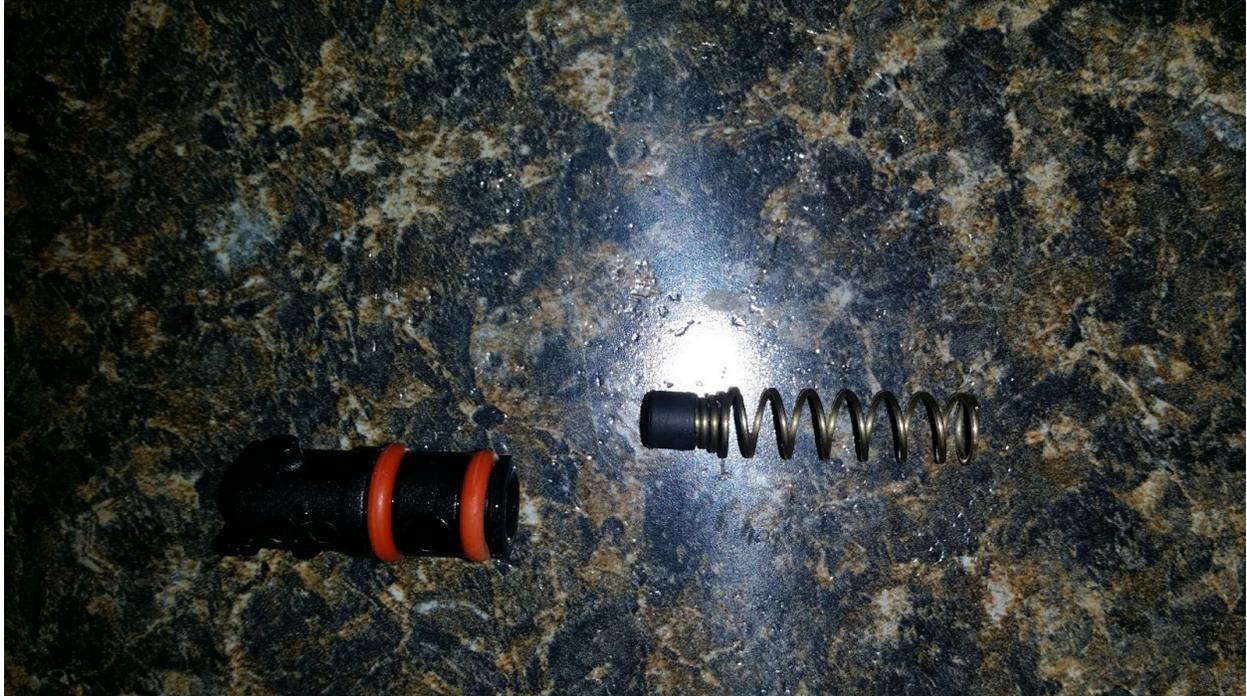
The little black plug you see in the photo is what causes the squeak. As it moves back and forth from the water pressure during the brewing process, it rubs against the inside of the plastic chamber.
