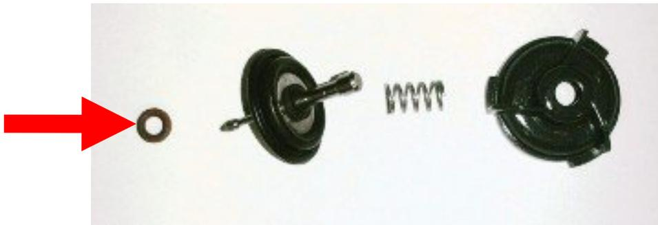
5. Remove the spring and set it aside. Grabbing it by the widest end, slowly pull the stainless steel post out. Be advised, this part is attached to the rubber disc (pictured). If it is dirty or has not been removed before, it may require some force. Be careful to pull strongly, but **slowly**.
