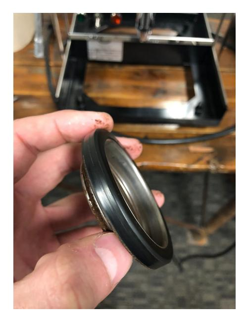
You can see in the picture above the lip that we referred to previously. You can also see how the gasket holds the shower screen onto the group. The gasket goes around the shower screen, against the lip, and then holds everything into the group with the friction from the gasket. Take this time to clean off your shower screen, soak it if it has a good degree of build-up, and once clean, put the gasket back over the shower screen.
