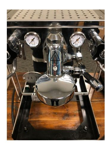
Your group gasket is located up in the head of the machine, where you lock in your portafilter. If you have the standard rubber gasket, it should just be a thick, black gasket:
