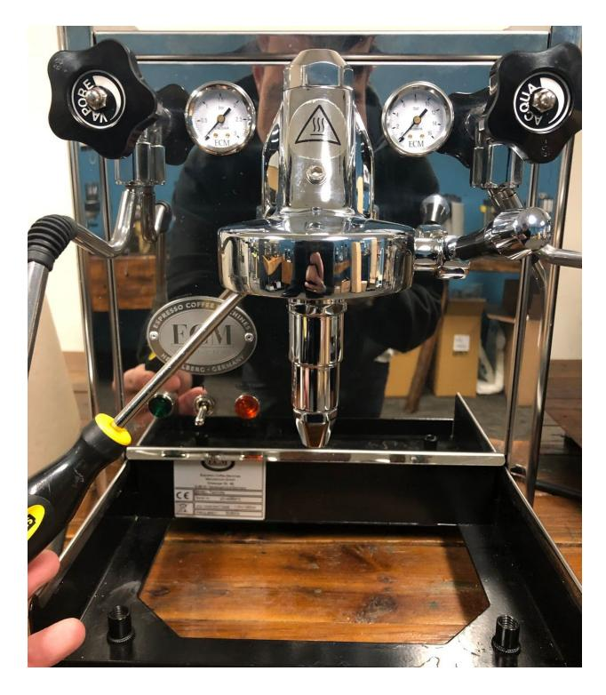
Place the end of the flathead on the small lip that runs around the diameter of the shower screen. Pry in one spot, and then move to another and pry again. Similar to the way you would open a paint can.
