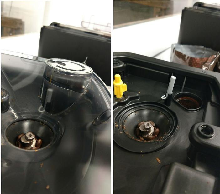
3. Remove the black screws that secure the top to the side housing panels. This will allow you to remove the plastic plate covering the grinder and access the grinder assembly. Take care to avoid lifting the panel far enough that the sensor wire is pulled or tugged, ensure that wire remains slack.
