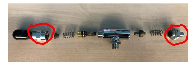
Once you have opened the valve, you should have the same parts and pieces that are laid out in this picture. Here's where you want to start inspecting for build-up. You can scrub down or try to clean off any visible or built-up scale on the springs and valving itself. If you're experiencing a sticky handle, the internal valve pin may need to be lubricated. You can apply some food-safe silicone grease to the part in the picture right:
