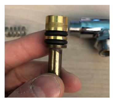
If this part is lacking lubrication, the valve can stick, or be slow to close - it could possibly even cause leaking if
