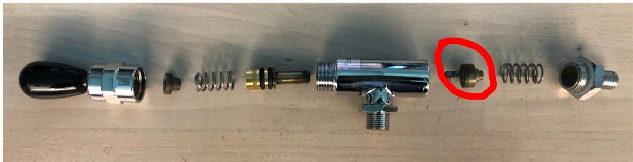
If it has signs of wear, you may want to replace it, that o-ring being worn can result in leaking.
