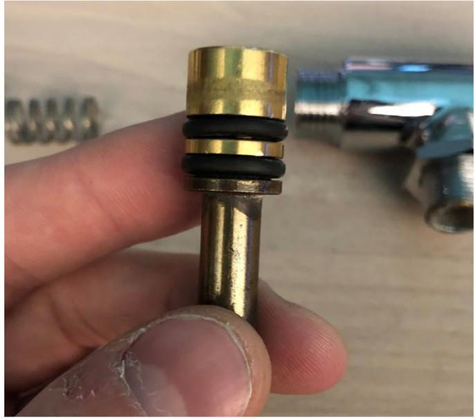
If this part is lacking lubrication, the valve can stick, or be slow to close - it could possibly even cause leaking if stuck open. You can spread the lubrication around the o-rings on the valve pin.
