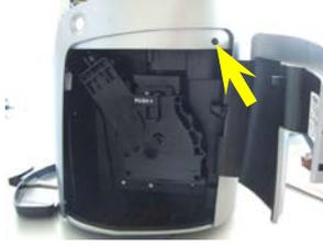
To remove the right side, loosen the screws as indicated.
