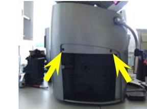
To remove the left side, loosen the screws as indicated.
