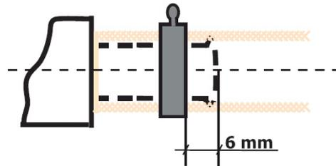
Figure (2) shows the assembly position of the clamp on the plastic solenoid pilot connectors.
