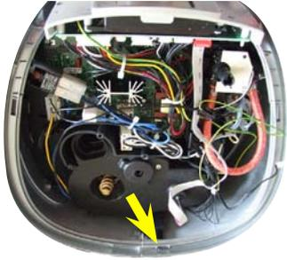
Loosen the screw as shown.
