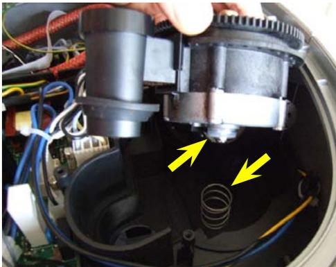
When refitting the motor assembly, be careful to reinsert the spring.
