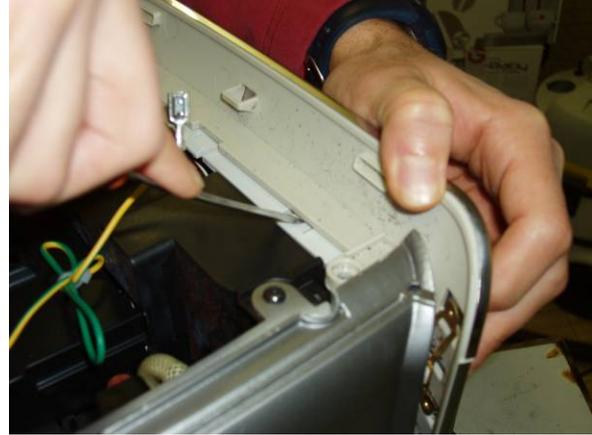
Unhook the anterior riser, by unblocking firstly the two lower hooks and then the upper ones ( see photo ), paying attention to not break the riser's hooks. After having removed the riser, it is possible to remove the frontal panel.
