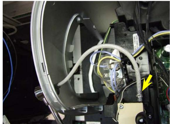
To take the left-side off, release the small clamp and pull out the wire mesh pipe connecting the steam pipe to the valve, removing the metal band as shown.
