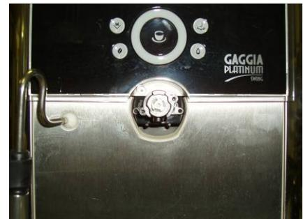
In order to dismantle the distributor completely, extract the regulation stick and, following the screws sequence, dismantle the different parts.
