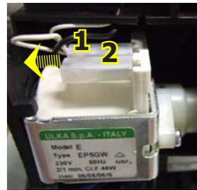
Withdraw the fastener connectors as indicated.
