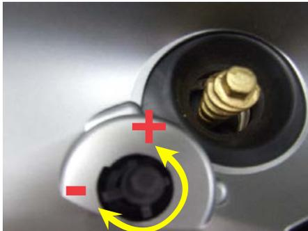
To vary the grinding setting, tighten or loosen with wrench "A" supplied.
