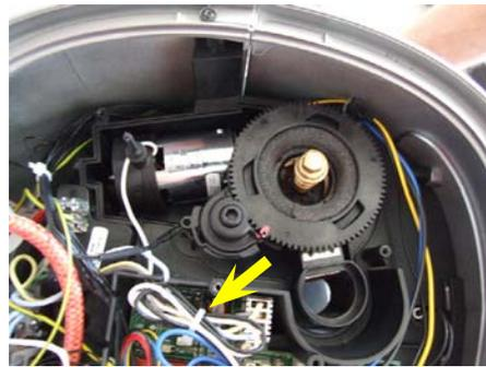
Unclamp and remove the connector inserted in the card.
