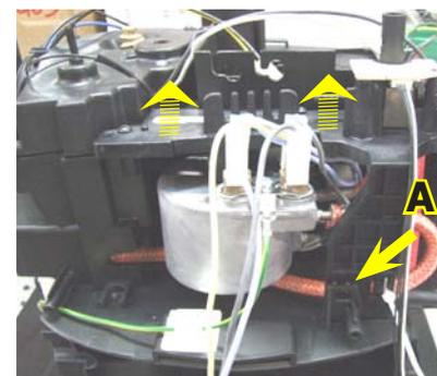
Unhook the teeth anchoring to the body and lift the heater and solenoid pilot.
