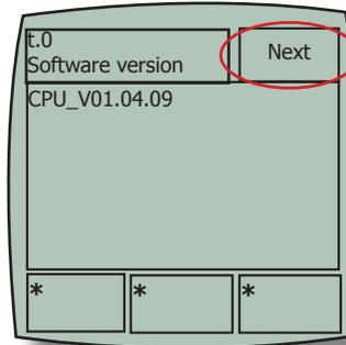
On entering test mode, the screen shown in the screenshot opens. Press the next key to move on to subsequent levels.
