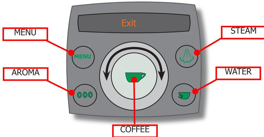
To move from one test level to another, use the touch-ring around the coffee key, turning it clockwise to move to the next level and anticlockwise to go back a level. Press the coffee key to open the sub-menus. Press the coffee again to confirm any changes. Press the menu key to exit sub-menus.
