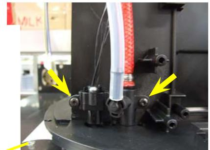
Loosen the screws on the relief valve assembly.
