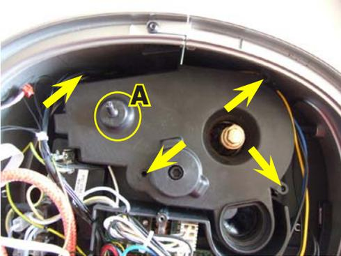
Loosen the screws on the cover and lift it off, being careful to withdraw damper A.
