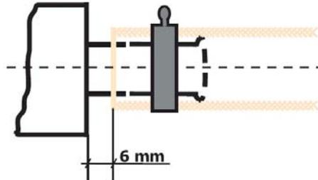
Figure (1) shows the assembly position of the clamp on the heater connector.
