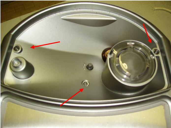
Remove the coffee top container, unscrew the three screws pointed out and lift the upper cover.
