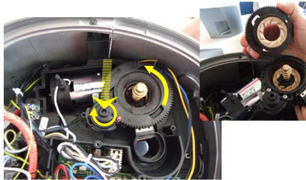
To remove the upper grinder support, use a wrench, turning it clockwise to release the grinder support from the bayonet coupling.
