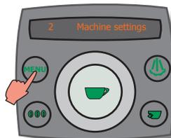
To exit at any time from "Machine settings" without saving any changes made, press the MENU key.
