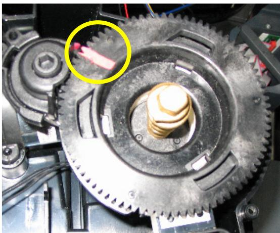
When refitting the upper grinder support, take care to reposition the mark as shown in the picture.
