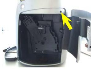
To remove the right side, loosen the screws as indicated.
