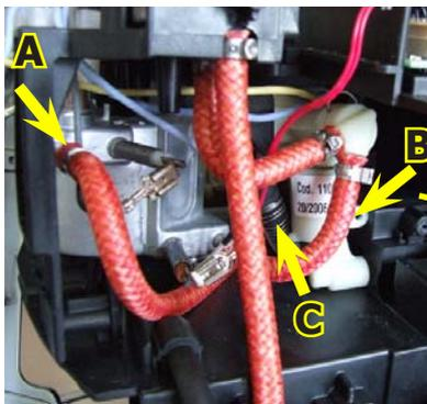
Take off the oetiker clamp A, pull out the reinforced flexible hose, loosen screw B and withdraw the drain pipe C from the solenoid pilot.
