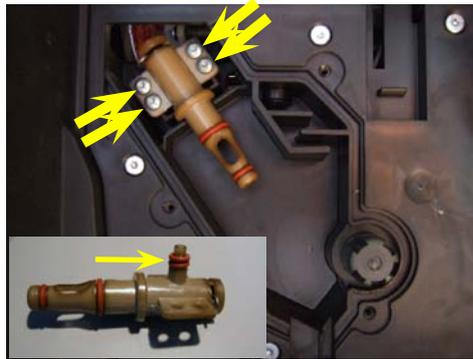
Loosen the four screws indicated and remove the heater valve asm. When refitting it, be careful with the two oil-rings shown in the smaller picture.
