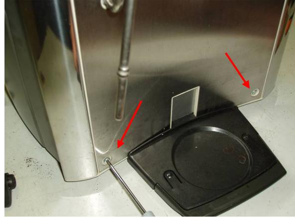
Unscrew the four screws which block the frontal panel, so that it can move.
