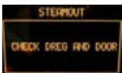
**IMPORTANT NOTE:** to execute the Steam-Out procedure the DREGDRAWER must be in place and the DOOR must be closed. If these 2 conditions are not respected a warning message is shown on the display and the Steam-Out is interrupted.
