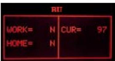
**ERROR:** The indication WORK doesn't change and remain "N", the display backlight changes from green to red; Check the work microswitch (broken?), the BU motor (blocked?) and the wiring (JP16).
