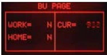
**ERROR:** (With BU) The absorbed current is more than 300mA, the display backlight changes from green to red; check the BU and the motor
