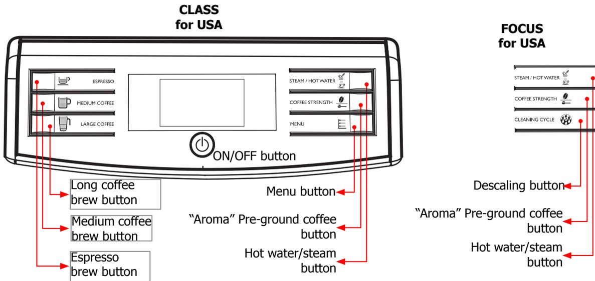
This machine is equipped with a colour-coded system to make your understanding of the display signals easier.
