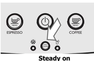
The machine needs to be descaled. Follow the steps described in the "Descaling" chapter of this manual.
