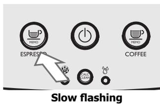
The machine is brewing one cup of espresso.
