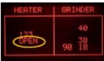
**ERROR:** In the indication HEATER appears "OPEN", the NTC temperature-sensor is detached or broken, the display backlight changes from green to red; check the wiring from the NTC temperature-sensor to the CPU/POWER board (JP13).
