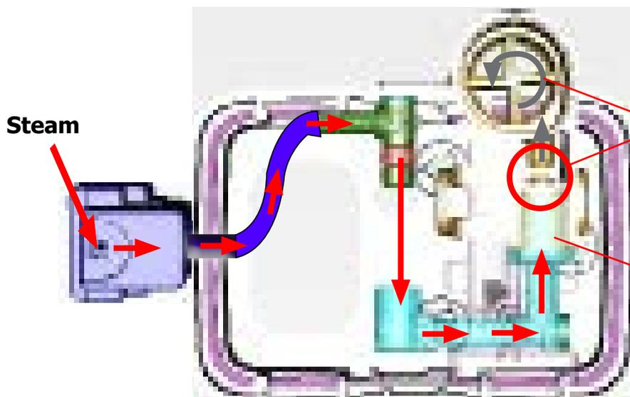
The milk is heated by the steam and taken towards the emulsion chamber where it is mixed with air and transformed into foam
