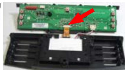
Disconnect the electrical connections.
