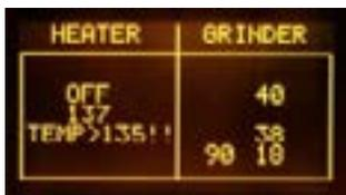
**ERROR:** the absorbed current is KO or the temperature does not increase; check the wiring from the heater to the CPU/POWER board (JP19) and the wiring of the NTC temperature-sensor (JP13).
