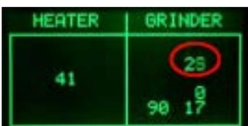
The grinder rotates and in the indication GRINDER the number increasing up to 40. The other numbers inside the GRINDER box are not important for this test.
