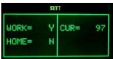
When the BU reaches the work position the indication WORK changes from "N" to "Y", the number of the current is minus than 200mA (without BU) or 300mA (with BU).
