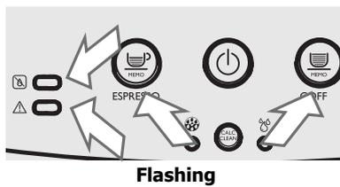
The machine is priming the circuit.
