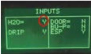
ERROR: The indication TANK-H2O doesn't change; check the capacitive sensor (fixing) and the wiring (JP23)
