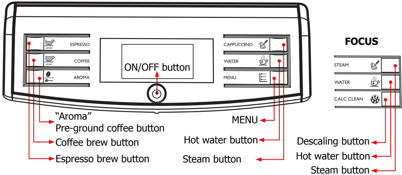
This machine is equipped with a colour-coded system to make your understanding of the display signals easier.
