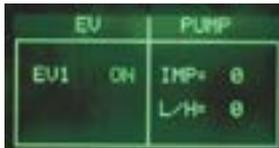
It is possible to hear the "click" from Electro Valve. The indication beside the **EV1** changes from "OFF" to "ON".
