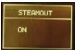
The machine starts the Steam Out and the display change the backlight (yellow) and appears the indication "ON". While the Steam Out runs the Electrovalve is opened and water comes out the Water/Steam pipe.
