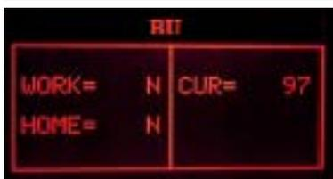
**ERROR:** The indication WORK doesn't change and remain "N", the display backlight changes from green to red; Check the work microswitch (broken?), the BU motor (blocked?) and the wiring (JP16).
