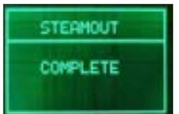
When the Steam Out is complete the message "COMPLETE" is shown on the Display. The Electrovalve automatically closes and the machine can be switched off.
