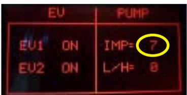
**ERROR:** The display backlight changes from green to red and the impulse remains 0; If water comes out the pipe: check the wiring from the flowmeter to the CPU/POWER board (JP5). If no water comes out the pipe: check the pump and the wiring from the pump to the CPU/POWER board (JP24).
