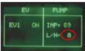
**ERROR:** The L/H is zero or very low; the Electro Valve does not open. Check the wiring from the Electro Valve to the CPU/POWER board (JP3) and the Electro Valve.
