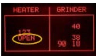
**ERROR:** In the indication HEATER appears "OPEN", the NTC temperature-sensor is detached or broken, the display backlight changes from green to red; check the wiring from the NTC temperature-sensor to the CPU/POWER board (JP13).
