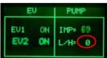
**ERROR:** The L/H is zero or very low; the Electro Valve does not open. Check the wiring from the Electro Valve to the CPU/POWER board (JP3) and the Electro Valve.
