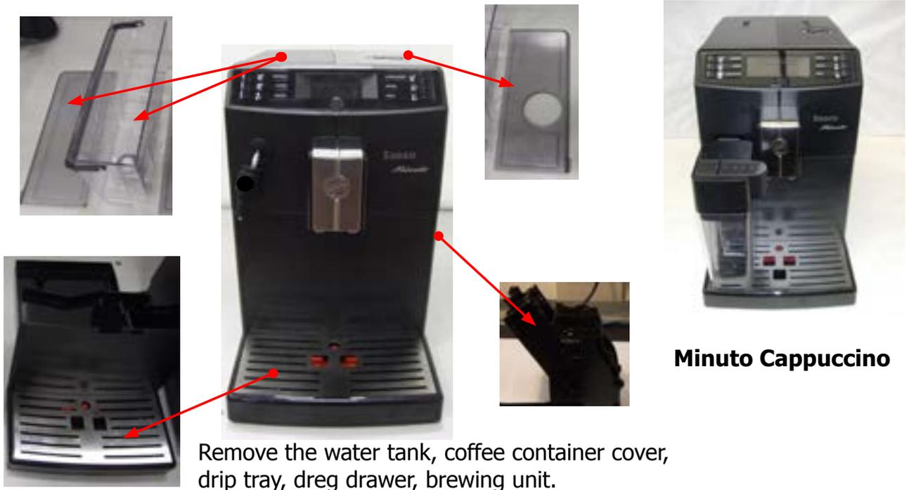
Remove the water tank, coffee container cover, drip tray, dreg drawer, brewing unit.
