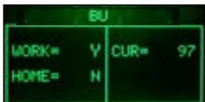
When the BU reaches the work position the indication **WORK** changes from "N" to "Y", the number of the current is minus than 200mA (without BU) or 300mA (with BU).
