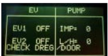
**Press the ESPRESSO button to open the Electro Valve 1**
