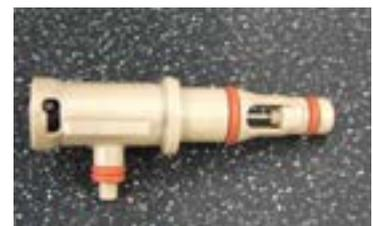
Loosen the screws as illustrated and remove the boiler pin (A).
