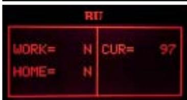
**ERROR:** The indication HOME doesn't change and remain "N", the display backlight changes from green to red; Check the work microswitch (is broken), the BU motor (is blocked) and the wiring (JP16).
