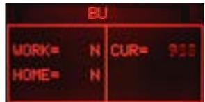
**ERROR: (With BU)** The absorbed current is more than 300mA, the display backlight changes from green to red; check the BU and the motor
