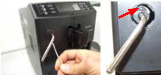
Remove the steam pipe cover as picture and unscrew the screw shown.
