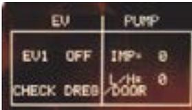
**Press the Z1 button to open the Electro Valve**
