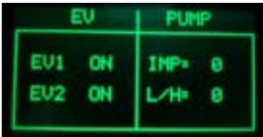
**Press the MEDIUM COFFEE button to open the Electro Valve 2**
