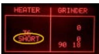
**ERROR:** In the indication HEATER appears "SHORT", the NTC temperature-sensor is shorted, the display backlight changes from green to red; check the wiring from the NTC temperature-sensor to the CPU/POWER board (JP13).
