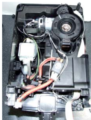
Remove the upper cover and remove the electrical and water circuit connections.
