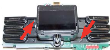
Loosen the screws for remove the cover.
