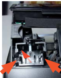
Loosen the screws holding the carafe connection
