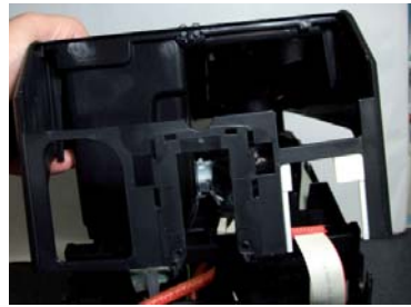
Remove the upper cover and remove the electrical and water circuit connections.
