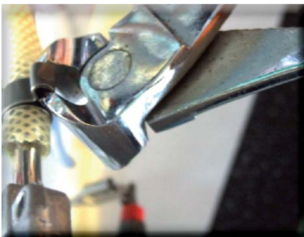
Use a suitable pair of pliers to remove the clamp (as illustrated).
