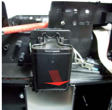
Unscrew the screws shown and remove the dispenser
