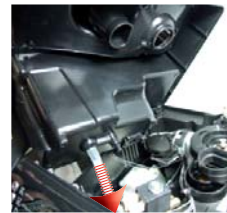
Remove the upper cover and remove the electrical and water circuit connections.
