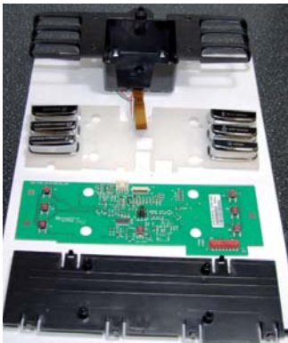
Remove the support KYB assy. and disconnect the flat cable.
