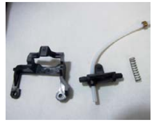
When reassembling the assembly to be careful to correctly position the spring.
